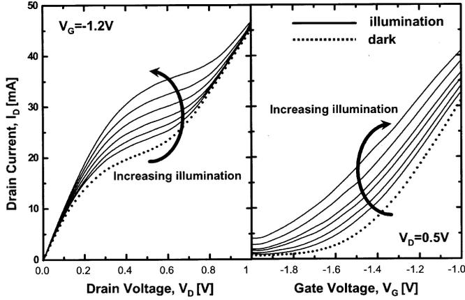
Fig. 2. Measured drain current ( $I_D$ ) as a function of drain voltage ( $V_D$ ) and gate voltage ( $V_G$ ) under 1.55- $\mu\text{m}$  optical illumination. The incident optical power increases from  $-12$  to  $3$  dBm with a 3-dBm increment.
