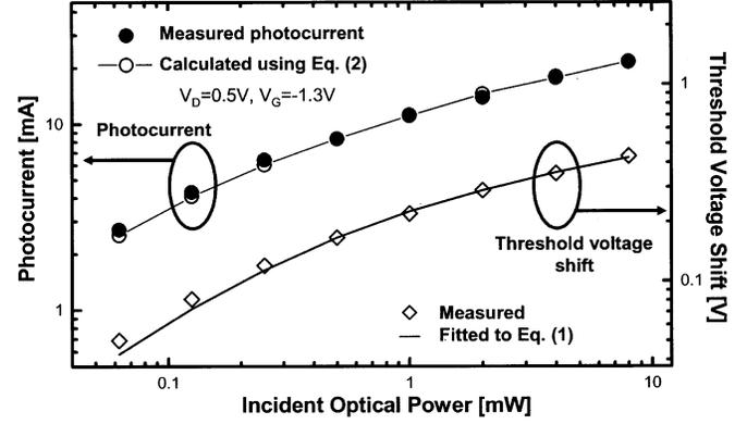
Fig. 3. Measured photocurrent ( $\bullet$ ) and the calculated increase in drain currents using (2) ( $-○-$ ) as a function of incident optical powers (upper curve). The measured threshold voltage shift ( $\diamond$ ) as a function of incident optical power; the line indicates the fitted data using (1) (lower curve). The gate bias condition of  $-1.3$  V was only used in the measurement of increased drain currents.
