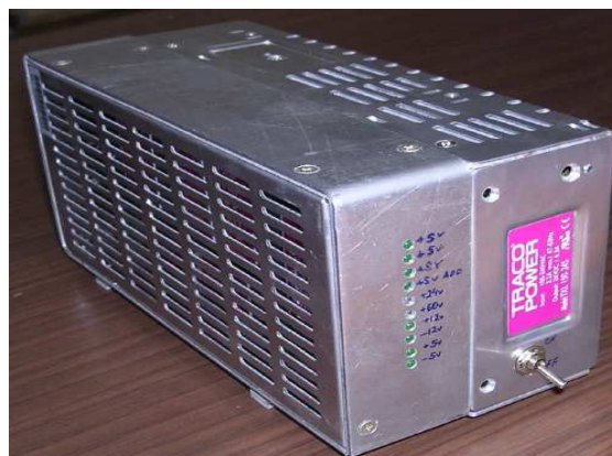
Fig 3.19 View of Power Supply Module
